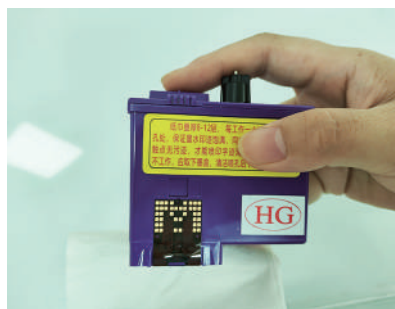
5. Take a piece of tissue and put it against the print head.
